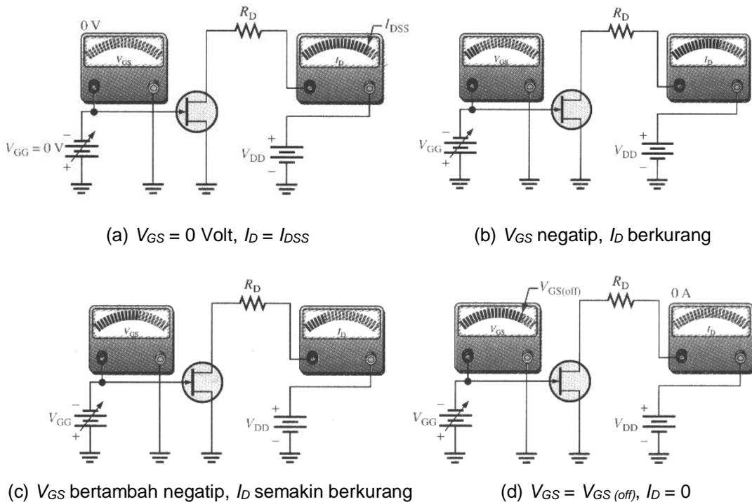
**Gambar 11.3 :**  $V_{GS}$  mengontrol  $I_D$
